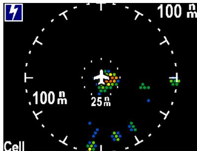
The display range of a thumbnail application is not adjustable with the *DATA/RNG* knob; however, the thumbnail application may be
