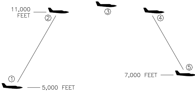
Figure 6 Example of Altitude Alerter Operation
