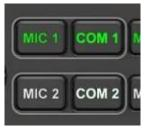
There are two pushbuttons associated with the transmitter selection. The two left buttons (MIC 1 & MIC 2) control which transceiver is selected for transmit. The right column of pushbuttons (COM 1 & COM 2) allows selection of the receiver audio. Push the MIC button to select the desired transmitter.
