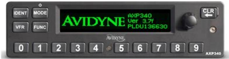
Following a successful power-on self-test, the AXP340 will transition to an operating mode and present the squawk code and Pressure Altitude display page.
