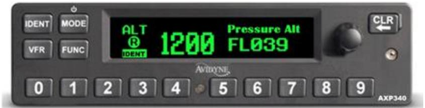
The AXP340 is a panel-mount Mode S transponder with support for 1090 MHz Automatic Dependent Surveillance Broadcast (ADS-B) Extended Squitter (ES), also known as “ADS-B Out” that meets all the requirements for Mode S elementary surveillance transponders for both IFR and VFR flight.
