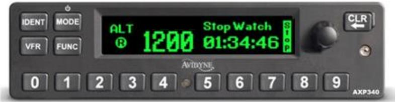
Press the FUNC button to display the stopwatch. Pressing the selector knob starts and stops the timer. Pressing the CLR button resets the timer.
