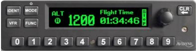
Pressing the CLR button resets the flight time counter. Pressing the selector knob starts or stops the flight timer. Pressing the FUNC button moves to the next screen and leaves the flight timer in the current state.
