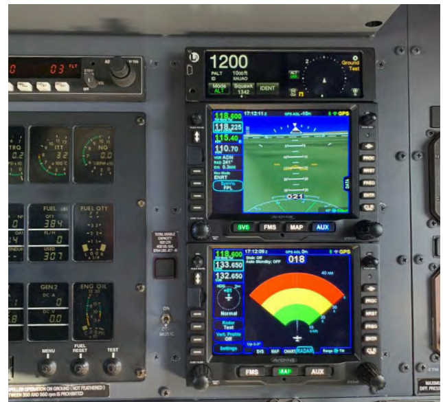
PC-12 installation with Lynx NGT9000, IFD550 and IFD540, AXP322 not shown
