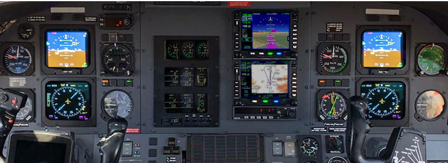
PC-12 installation with IFD550 and IFD540, NGT9000R, AXP322 not shown
