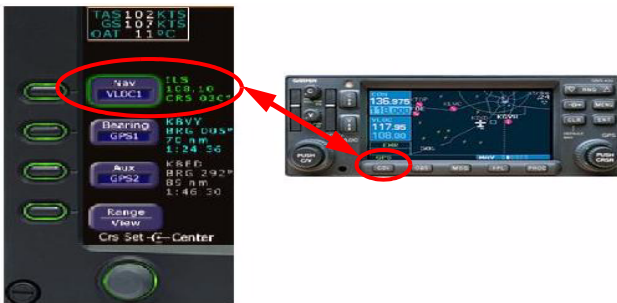
Figure 9. Setting CDI Scale on EXP5000's HSI
