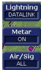
The Lightning and Traffic keys are not displayed if radar, lightning or traffic sensors are not installed. Instead, the METAR and AIR/SIG keys are displayed. These keys are On/Off switches of the respective features.
