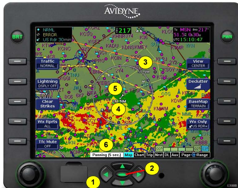
Figure 2.4 EX600 Panning Controls and Indications
