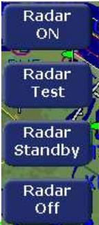
When Traffic and Lightning sensors are installed, only the main Radar key is available on the Map page. However, if fewer external sensors are installed, the EX500/EX600 takes advantage of the available keys. For example, if a second key is available for radar functions, a dedicated *Radar Off* key is displayed. Similarly, if other keys become free, additional radar keys display, including *Radar Test* and *Radar Standby*.
