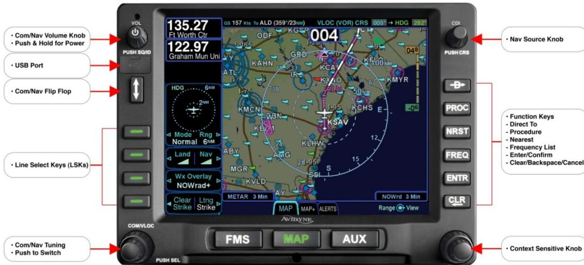
\*The IFD510 and IFD545 do not contain a VHF nav/com radio and therefore does not have a volume knob, flip/flop button, and Com/Nav push knob.
